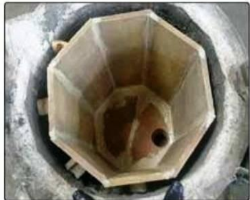
COLD BOARD LADLE LINING (This is with two bottom Boards and 8 nos vehicle Boards)
